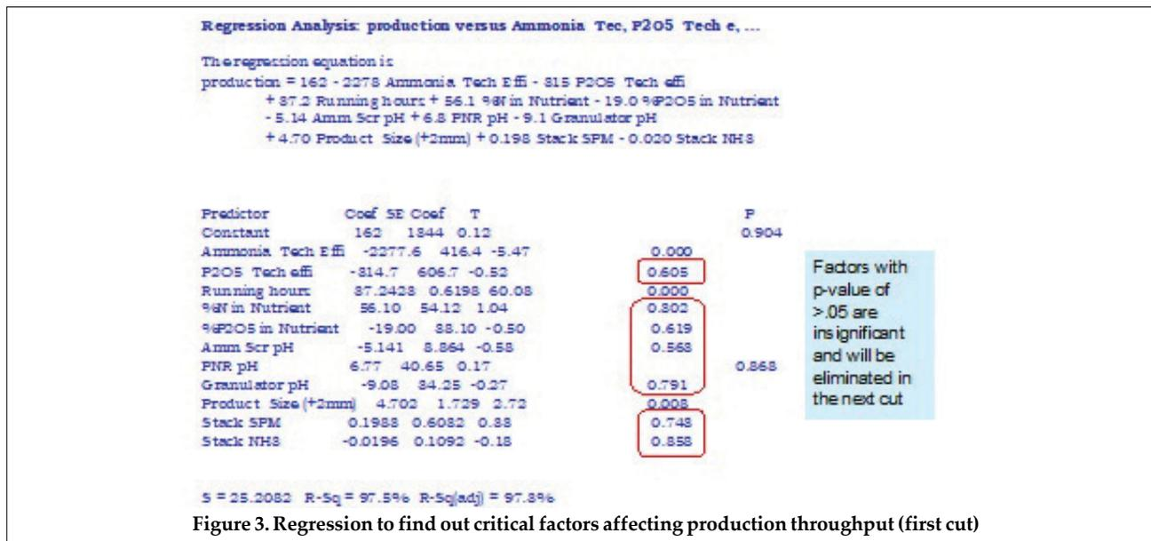
Figure 3. Regression to find out critical factors affecting production throughput (first cut)
