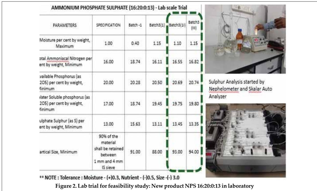
Figure 2. Lab trial for feasibility study: New product NPS 16:20:0:13 in laboratory
