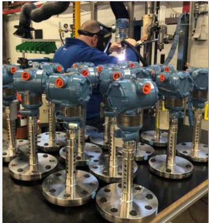
*Example of specialists' solution: a series of pressure transmitters with direct mounted blind flanged diaphragm seals with a temperature cooling option. This temperature cooling system reduces the elevated process temperature of up to 400°C to below the temperature limitations the pressure transmitter sensor can handle.*
