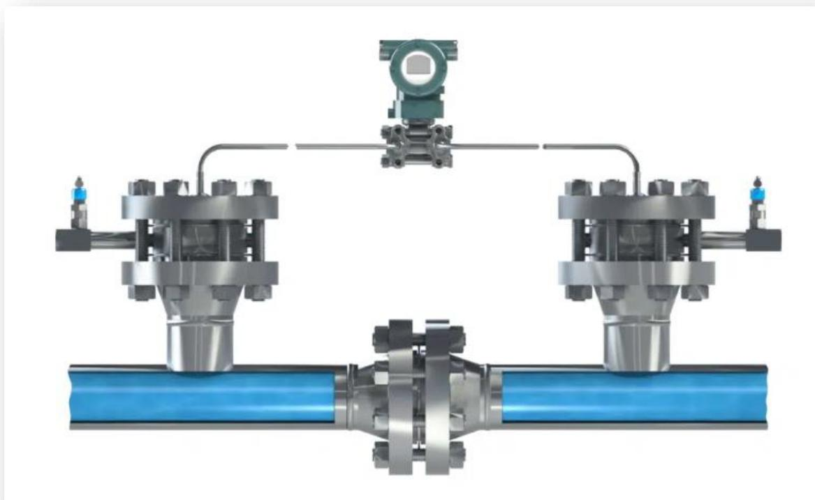
*Example of a slightly unusual way to use diaphragm seal systems: flow measurement by means of a differential pressure measurement. This is especially useful when there are elevated process temperatures or corrosive applications.*
