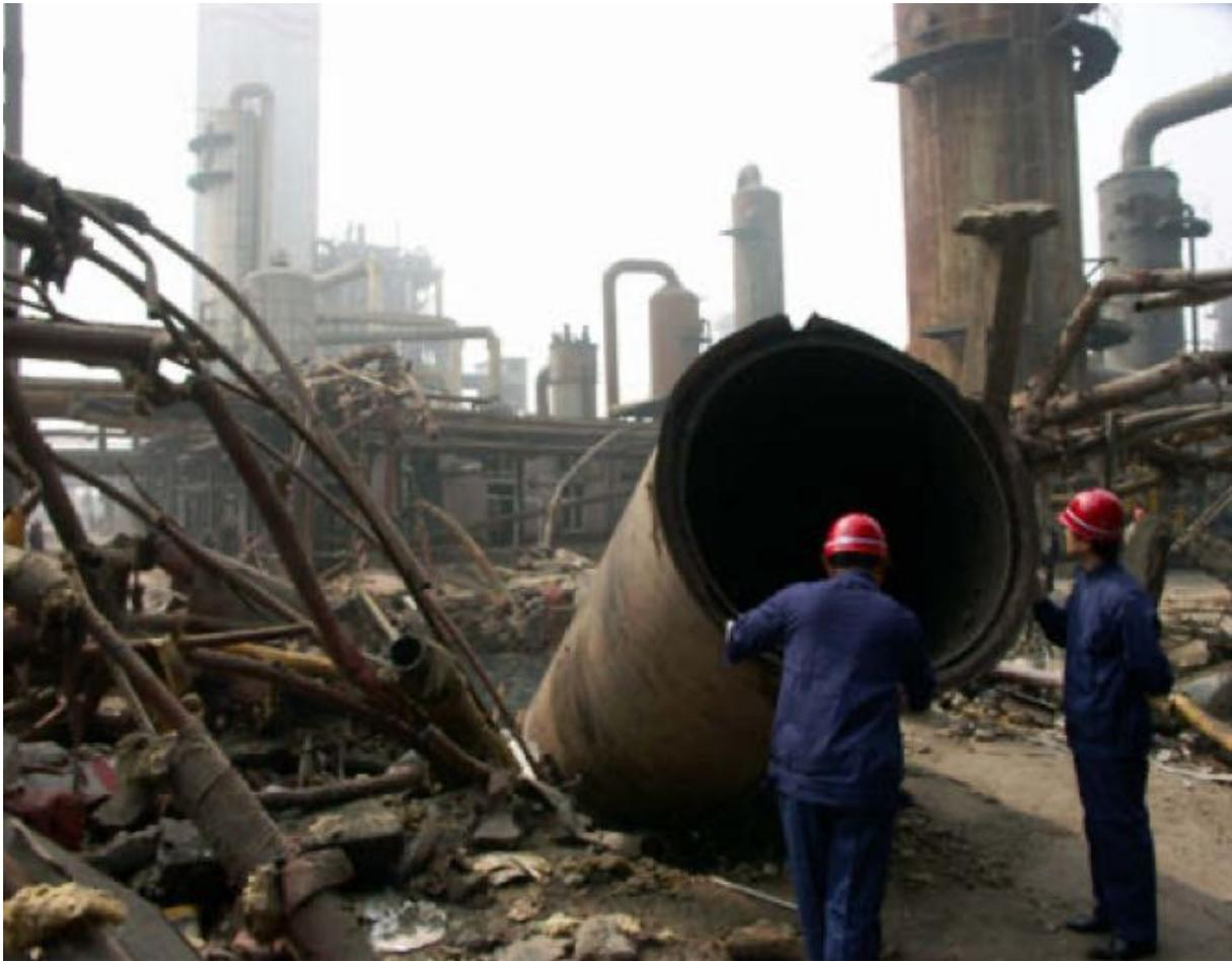
Figure 2: Rupture of a urea reactor (Incident 05-001)
