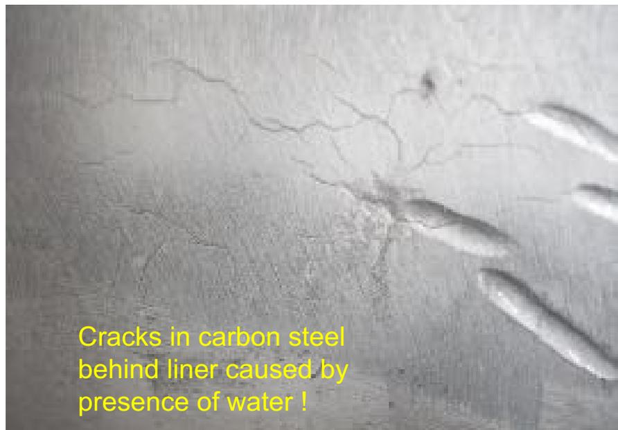
**Figure 1: Cracks in a carbon steel wall**
