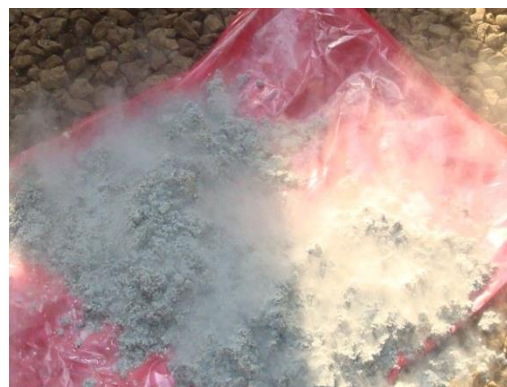
Fig (1) deposits from ammonia separator
