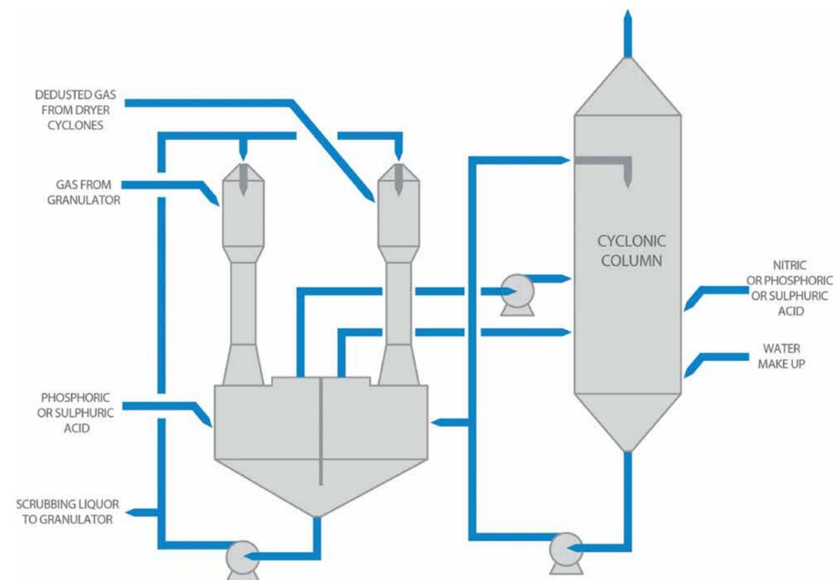
Figure 3. NPK granulation process
