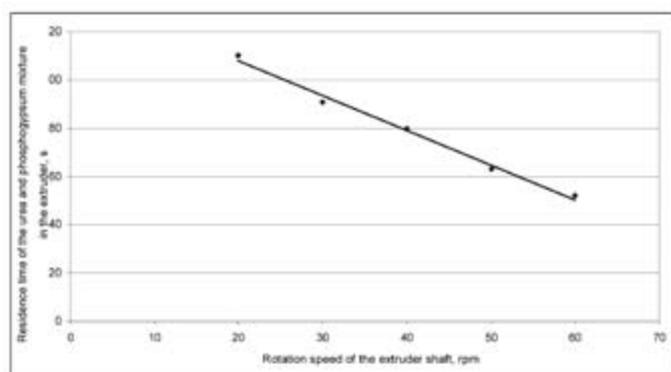
Fig. 3. Residence time of the urea and phosphogypsum mixture in the extruder
