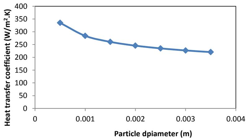
**Figure (5):** Effect of particle diameter on heat transfer coefficient.
