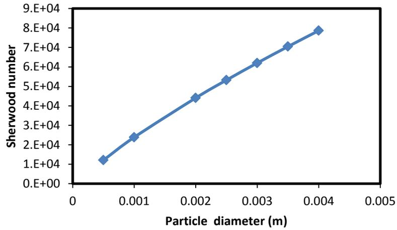
**Figure (6)** :variation of Sherwood number versus particle diameter.
