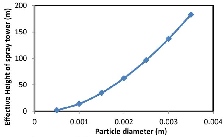
**Figure (4):** Effect of particle size on height of spray tower.
