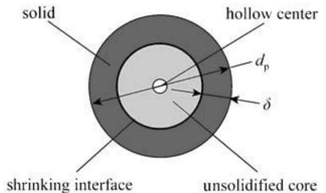
**Figure (2):** Shrinking unsolidified core model Wu *et al.* 2007.
