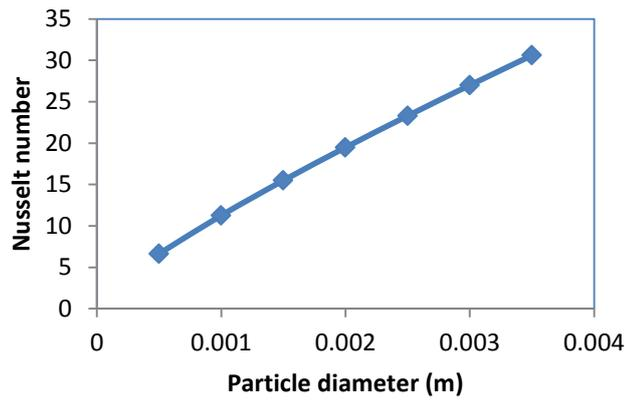
**Figure (3):** Effect of particle size on Nusselt number.
