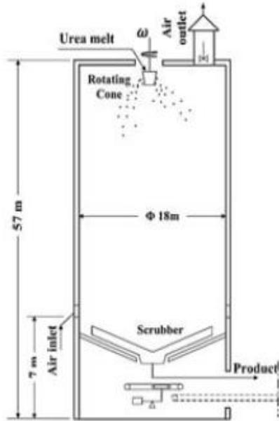
**Figure (1):** Schematic diagram for the Urea prilling tower. Ali Mehrez et.al (2012)
