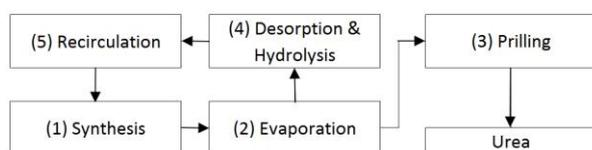
Fig.1 - Simplified block diagram for industrial urea production.
