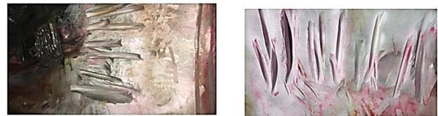
Figure 16. Grinded areas; at this location minimum remaining wall thickness is 10 mm
