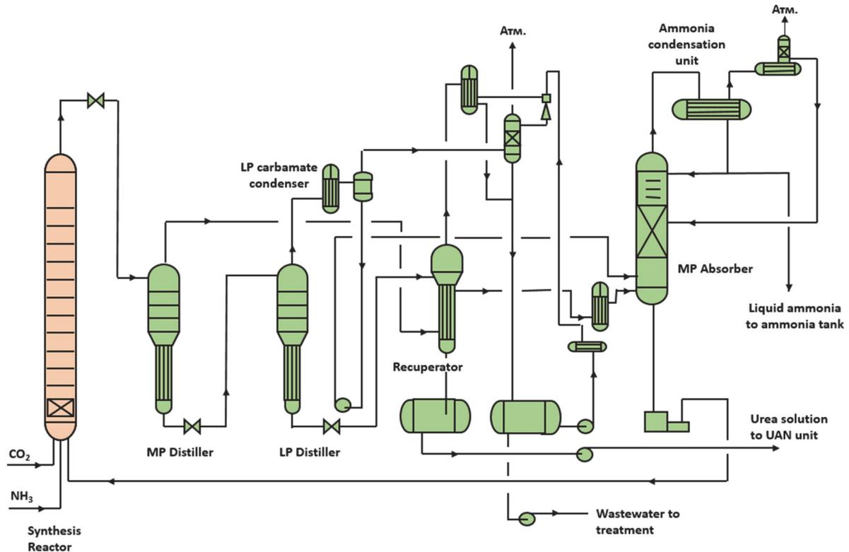
Fig. 3: PFD of URECON 2006® urea solution unit
