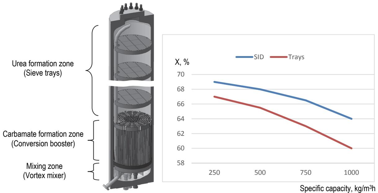
**Fig. 4: Efficiency upgrading of the urea synthesis reactor**
