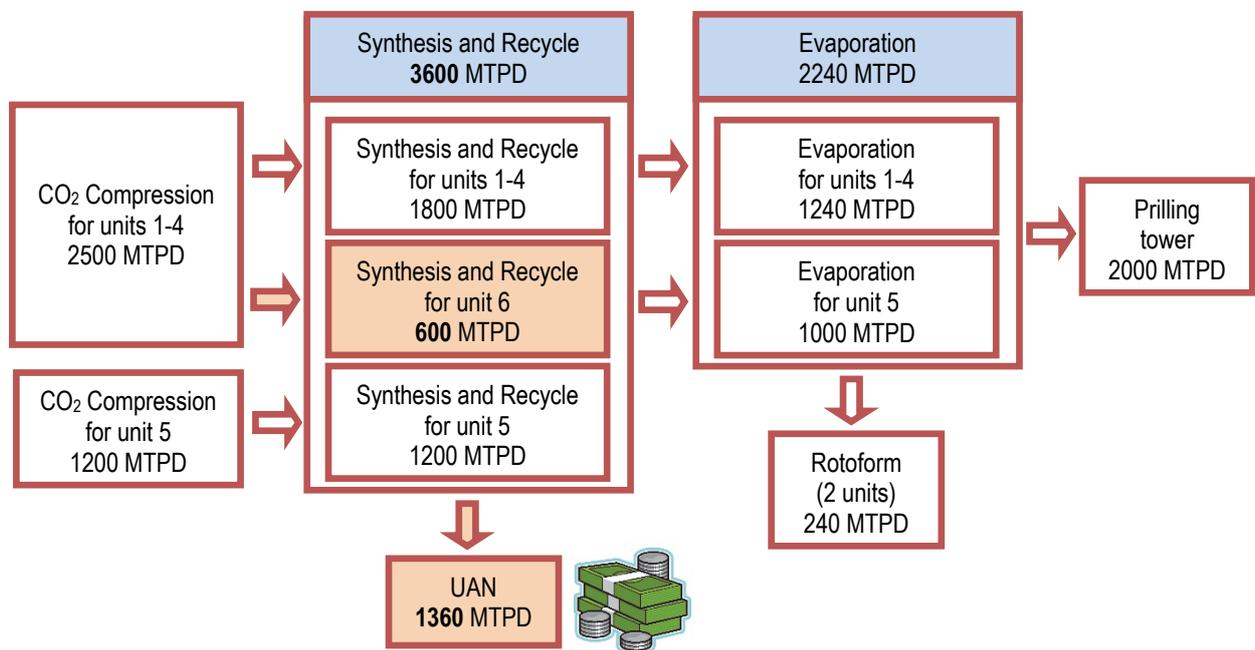
**Fig. 2: Block diagramm of urea production after enhancement**
