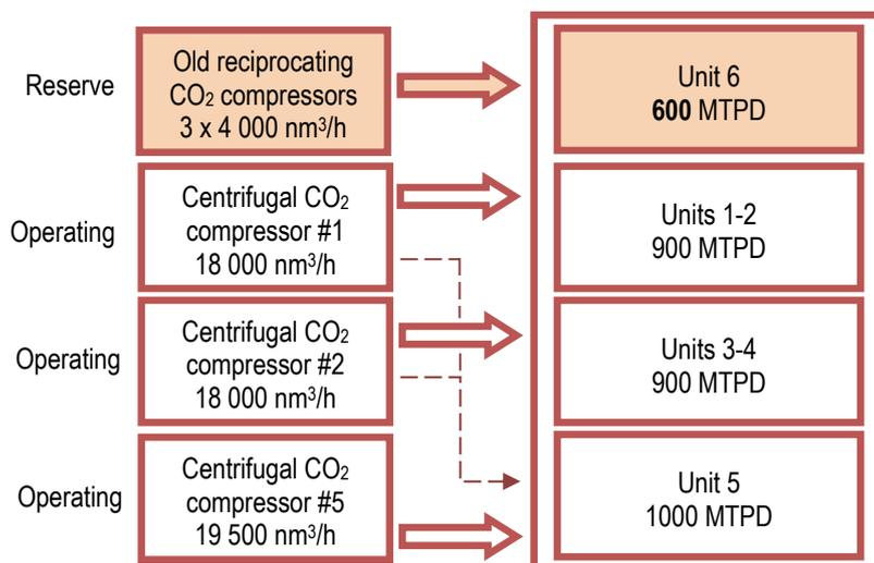
Fig. 5: Distribution of CO<sub>2</sub> compressors by urea plants
