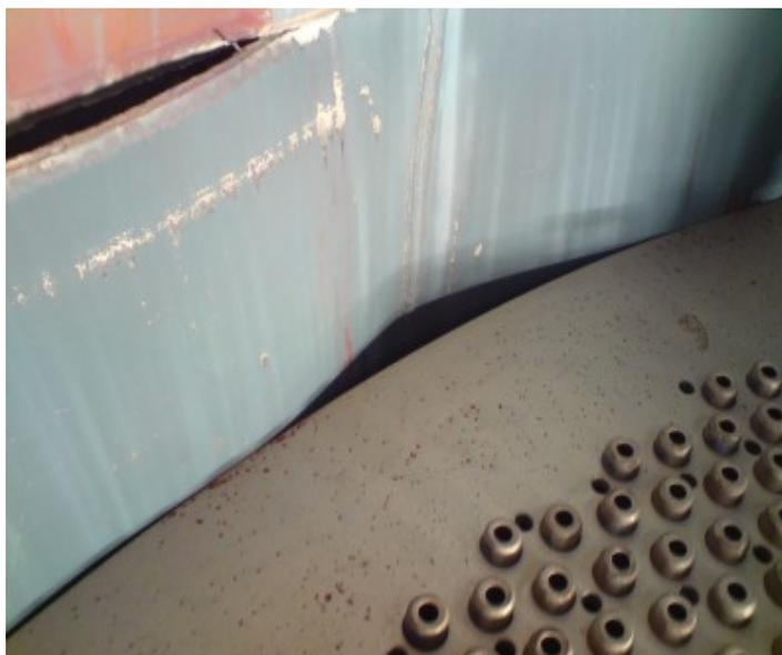
Figure 1 : Example of a bulged liner
