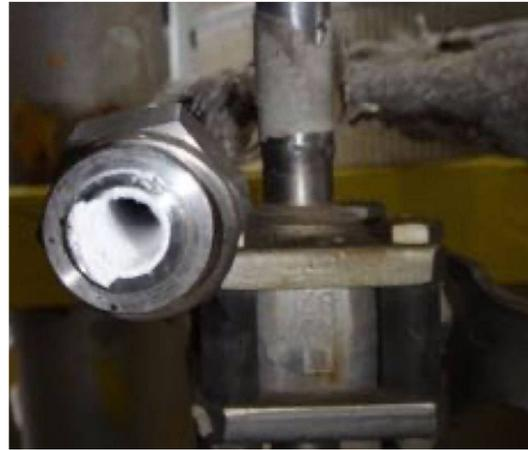
Pictures: Clogging behind a liner (left) and clogging of leak detection circuit tubing (right)
