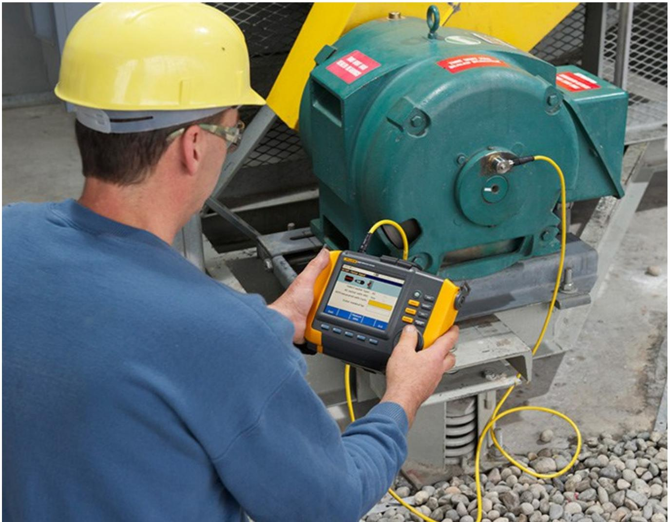
A technician uses a vibration tester on an operational motor. All images courtesy of Fluke Corporation
