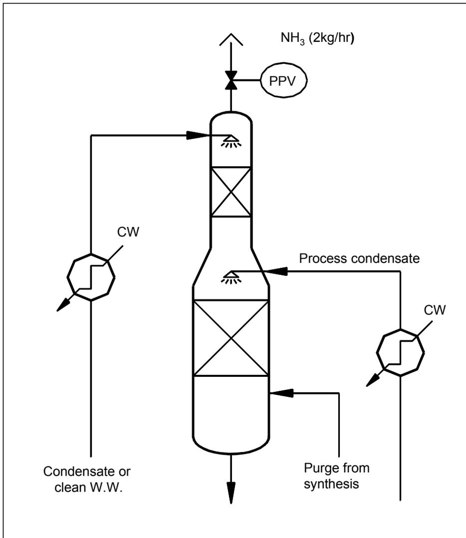
The total investment for a new 4 bar absorber system as indicated in Figure 1, which reduces the ammonia emission to less than 2 kg/hr, is estimated to be about 500.000 US\$ based on European conditions. This means that this project had a pay back time of less than 2 years, again based on European conditions.
