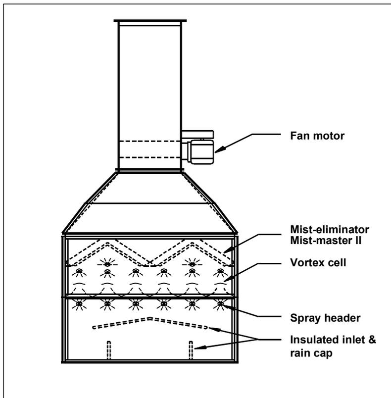
Air leaving the prill tower is hot and dry, while urea is hygroscopic. The relative humidity must be raised to the point where collected urea dust will absorb moisture and tend to liquefy.
