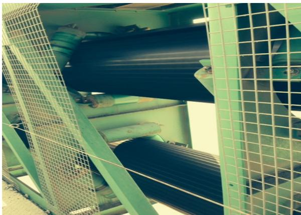
Figure 8 – Pipe Conveyors for Bulk Urea
