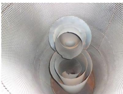
Figure 2 - damaged steam silencer
