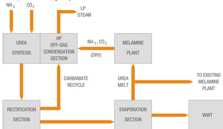
Fig. 5: Overall block diagram of Melamine and Urea units
