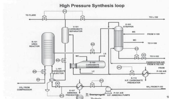
where the liquid Ammonia acts as a propellant for the high pressure Ammonium carbamate solution. CO<sub>2</sub> gas from compressor discharge at 158 bar and at 104!C temp enters into the Reactor.(Figure-02)
