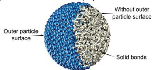
FIGURE 2. Agglomerate and its internal structure.
