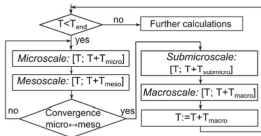
FIGURE 3. Flowchart of the main simulation algorithm.
