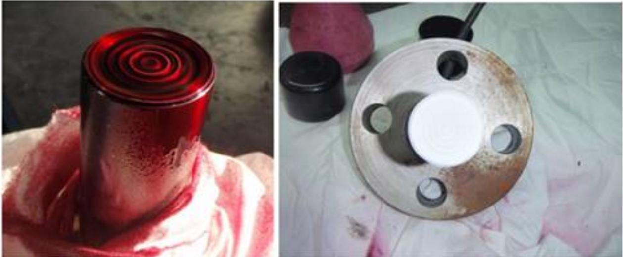
Dye penetrant test of diaphragms
