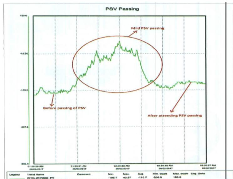
Figure 1: Pressure in discharge line before and during passing
