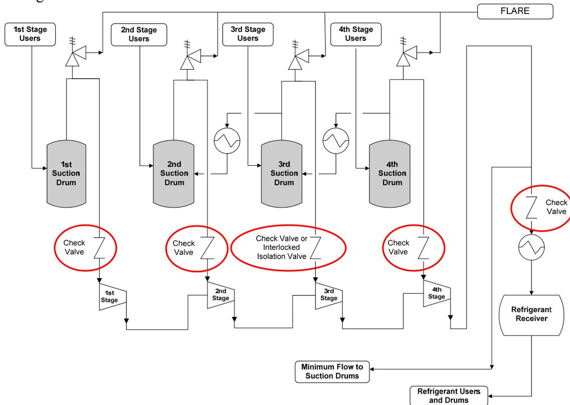
Limited interstage relief capacity has a relatively small impact on the magnitude of overpressure. However, due to the large 1<sup>st</sup> stage minimum flow valve capacity and large first-stage suction volume, low stage minimum flow valve response does have a significant impact on possible overpressure. Note, not all propylene refrigeration systems are designed with suction check valves or trip valves.
