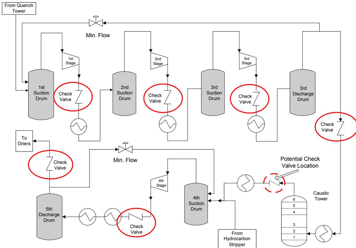
With check valves located at the discharge of each stage, overpressure hazards can exist at each stage for either individual or multiple check valve failure scenarios. Typically interstage relief capacity is relatively small, sized for a fire case scenario. Check valve failure can result in overpressure as high as 300% of MAWP.
