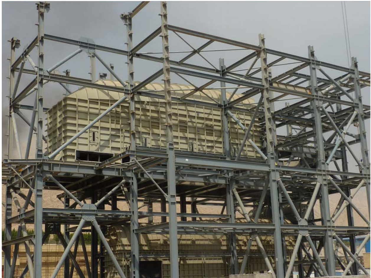
Figure 5: The Stamicarbon granulator with its optimized upper casing design.
