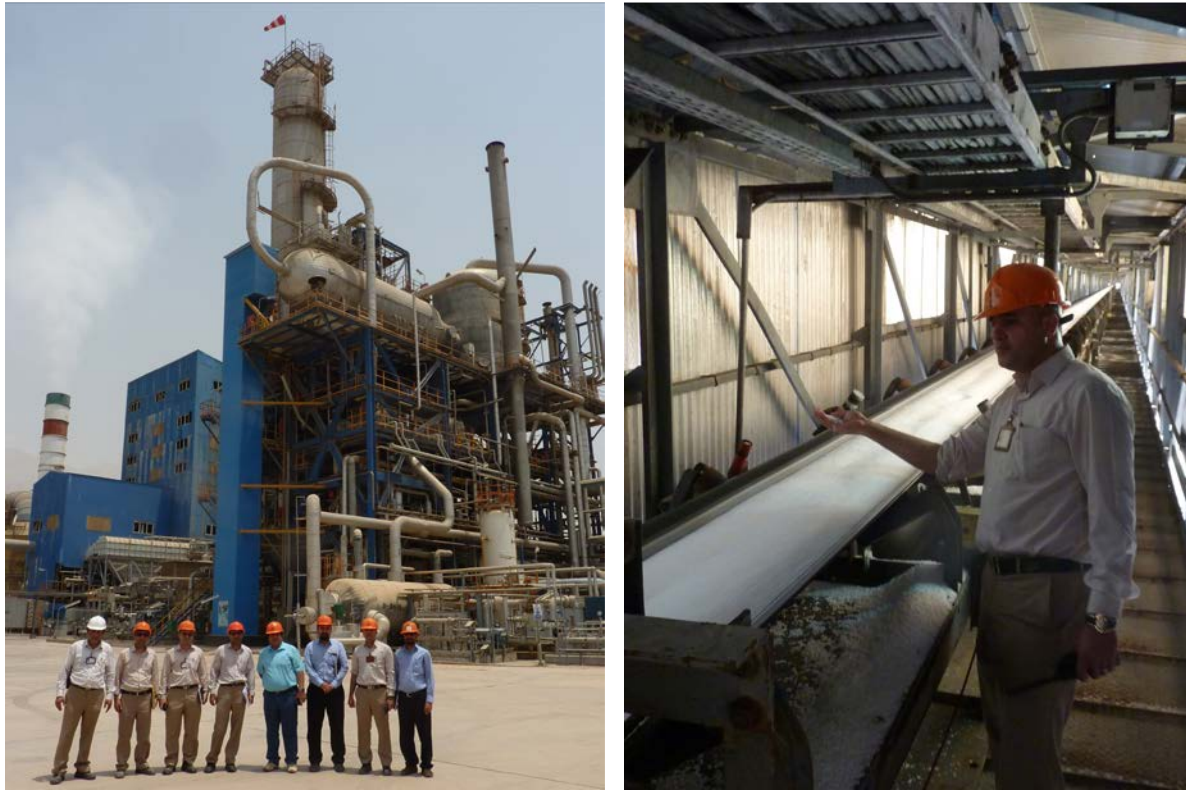
Figure 3: Pardis 1 Stamicarbon PoolCondenser urea plant and its perfect quality granular product.
