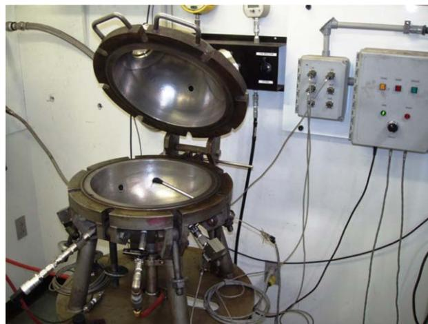
**Figure 3.** 20 liter test vessel. [Color figure can be viewed in the online issue, which is available at [wileyonlinelibrary.com](http://wileyonlinelibrary.com).]
