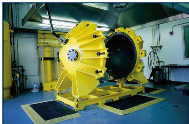
**Figure 2.** 1 Cubic meter test vessel. [Color figure can be viewed in the online issue, which is available at [wileyonlinelibrary.com](http://wileyonlinelibrary.com).]
