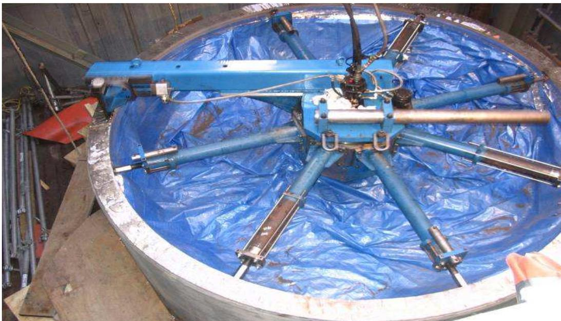
**Figure4: Machining of the weld preparation bevel**
