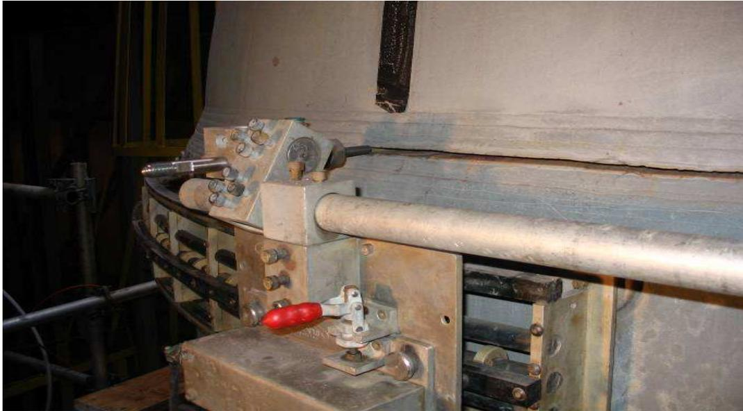
**Figure 3: Cutting of the head underway using HP water-jet / abrasive cutting**
