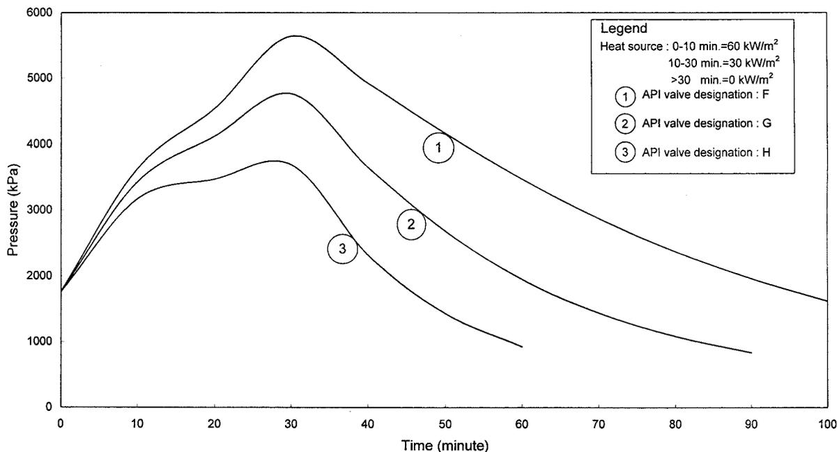
Figure 13. Effect of valve orifice on pressure versus time.
