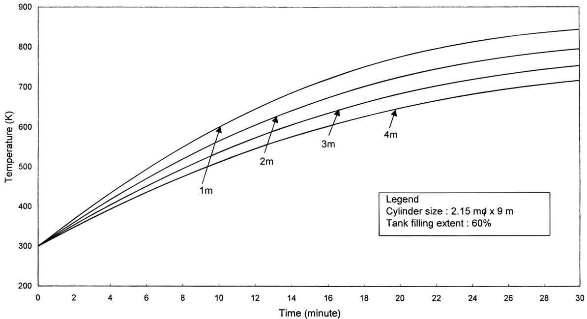
Figure 5. Effect of tank-to-tank spacing in case of a tank fire.
