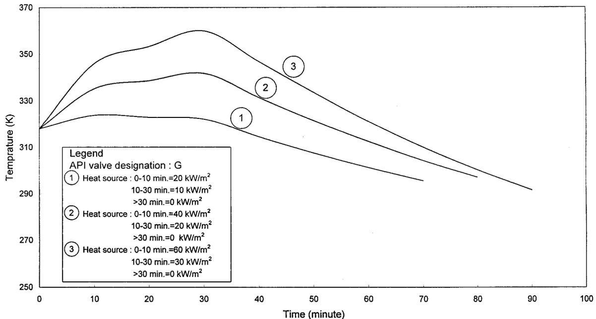
Figure 8. Temperature profiles versus time.
