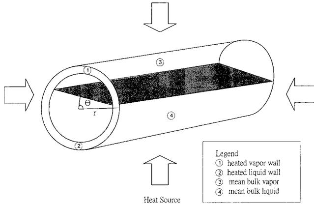
**Figure 1.** Four temperature nodes of a completely fire-engulfed horizontal tank.
