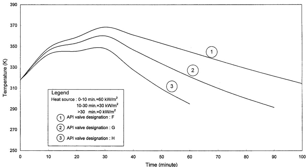
Figure 11. Effect of valve orifice on temperature versus time.
