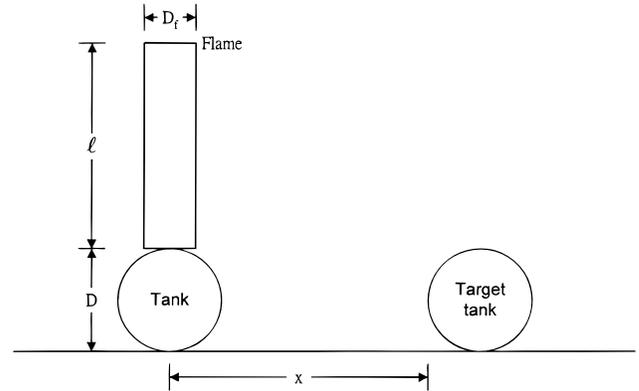
**Figure 2.** Solid flame model of a tank jet fire.
