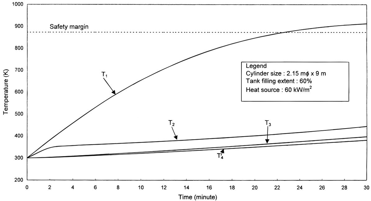
Figure 3. Profiles for four node temperatures at constant external heat.
