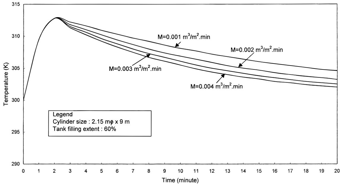
Figure 7. Variation in heated-vapor-wall temperature showing the effect of increasing amounts of water spray.
