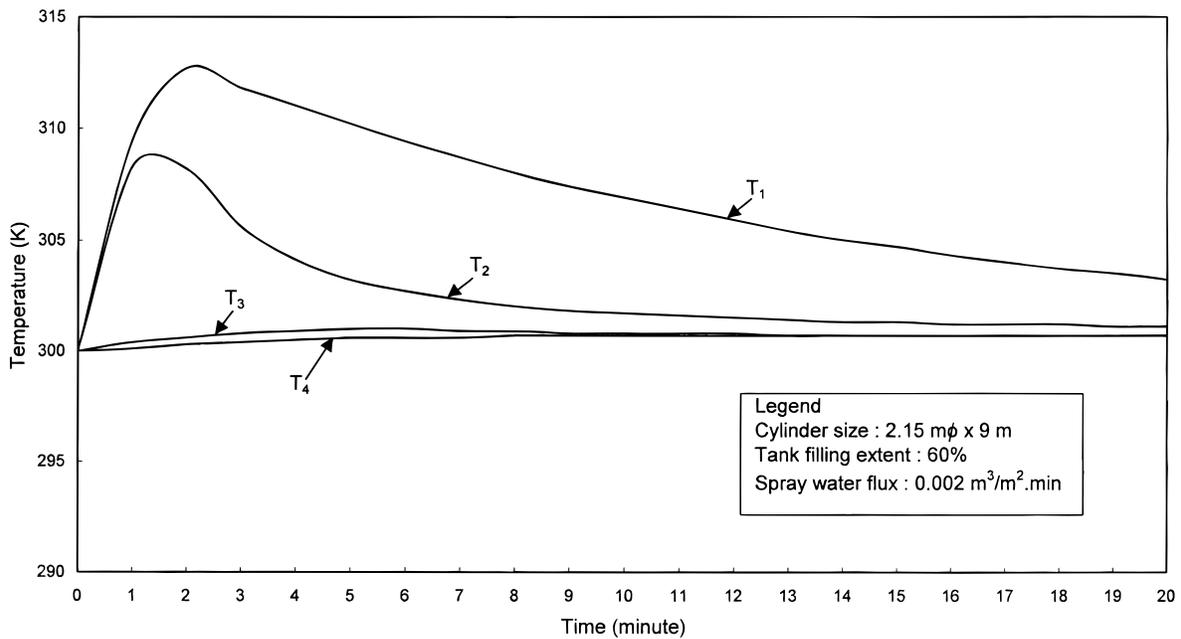
Figure 6. Variation in four node temperatures showing the effect of water spray.
