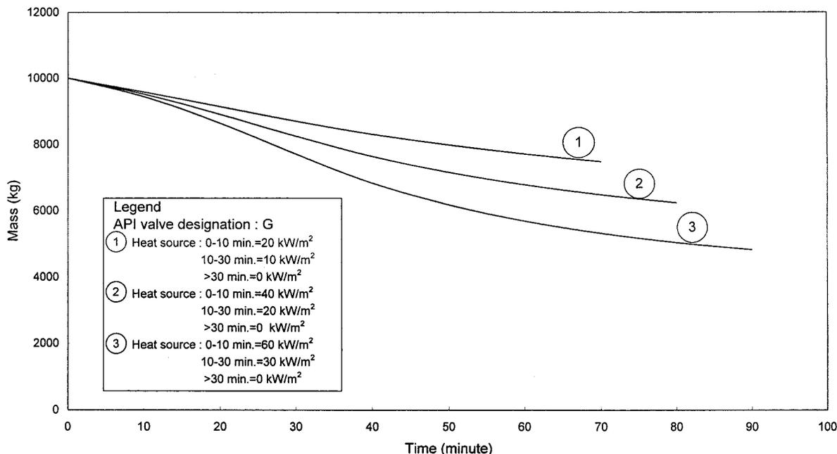
Figure 9. Profiles of tank liquid mass versus time.
