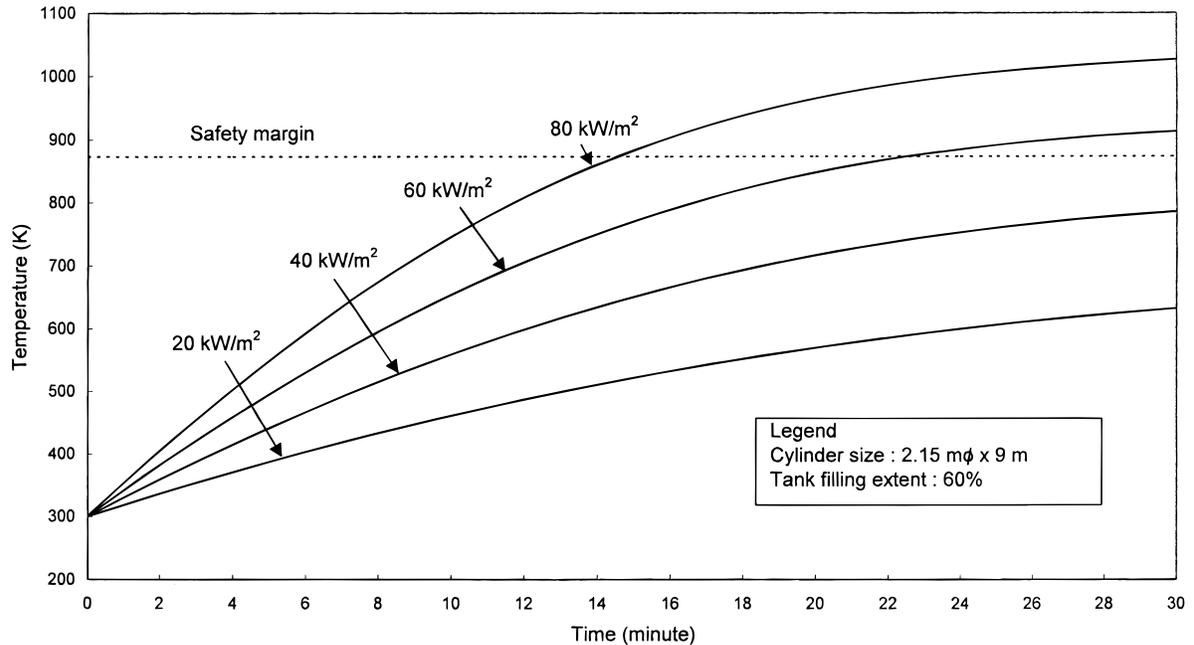
Figure 4. Variation in heated-vapor-wall temperature with varying external heat.
