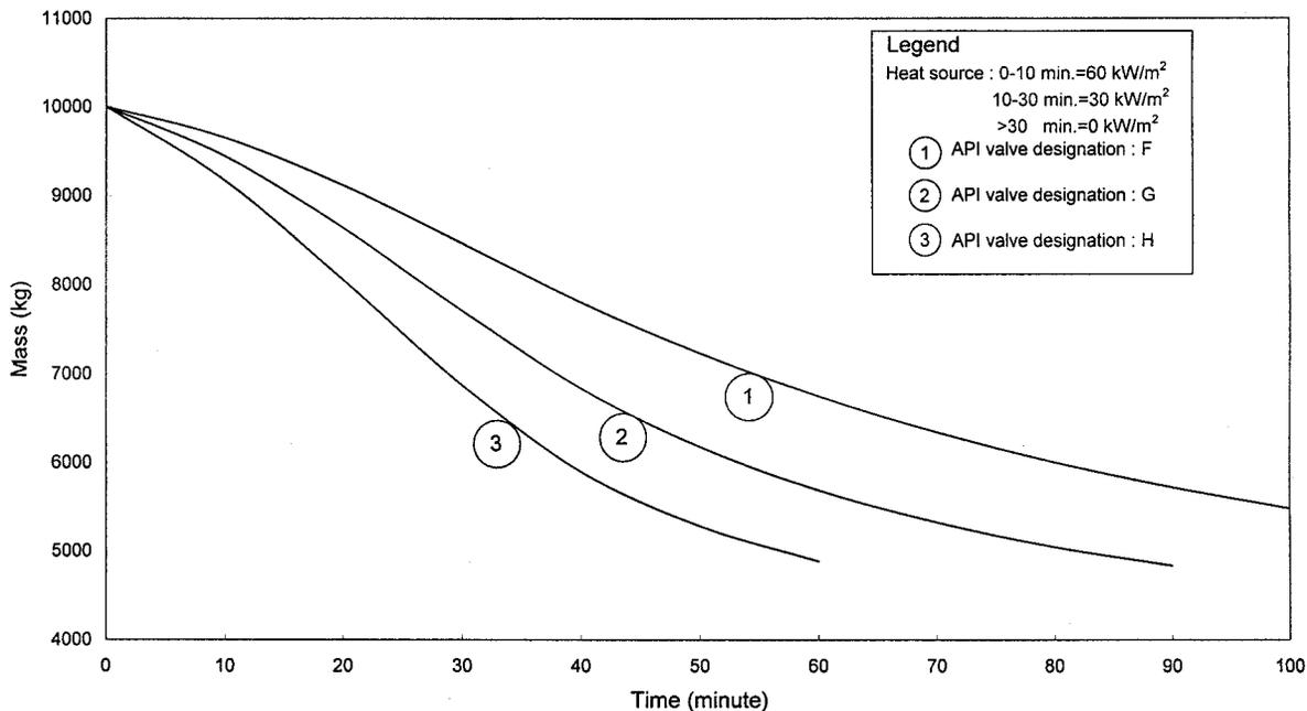
Figure 12. Effect of valve orifice on tank liquid mass versus time.
