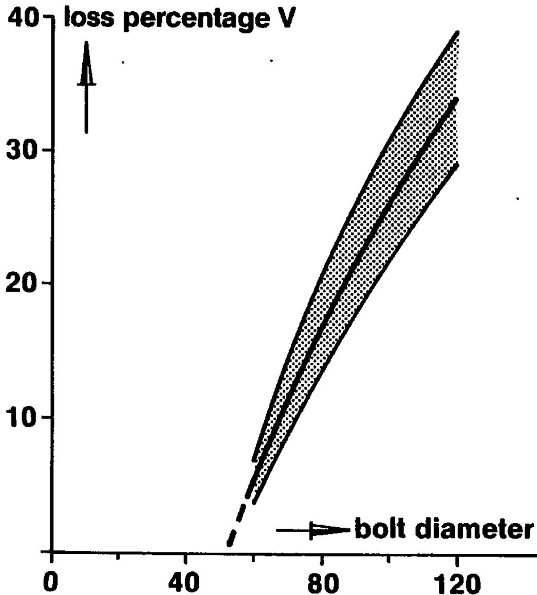
It indicates that the theoretically oil pressure of the hydraulic jack should be multiplied by a correction factor:
