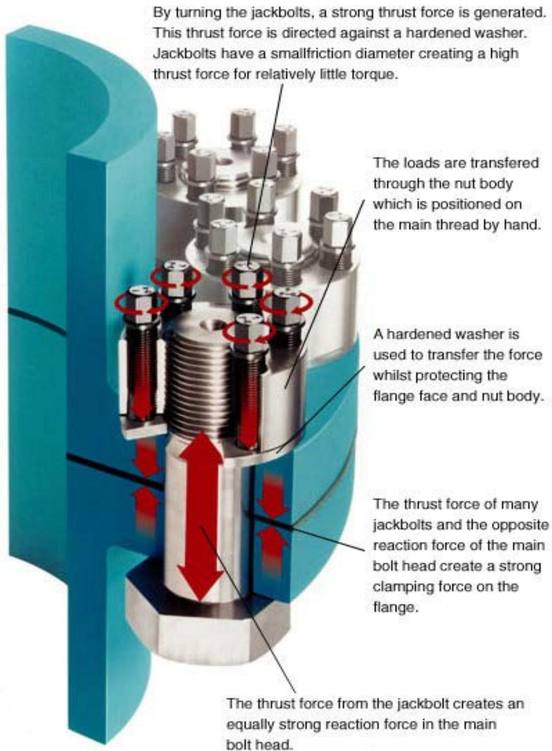
The procedure to follow is that at first the washer will be positioned and the round nut will be screwed hand tight onto the stud bolt.
