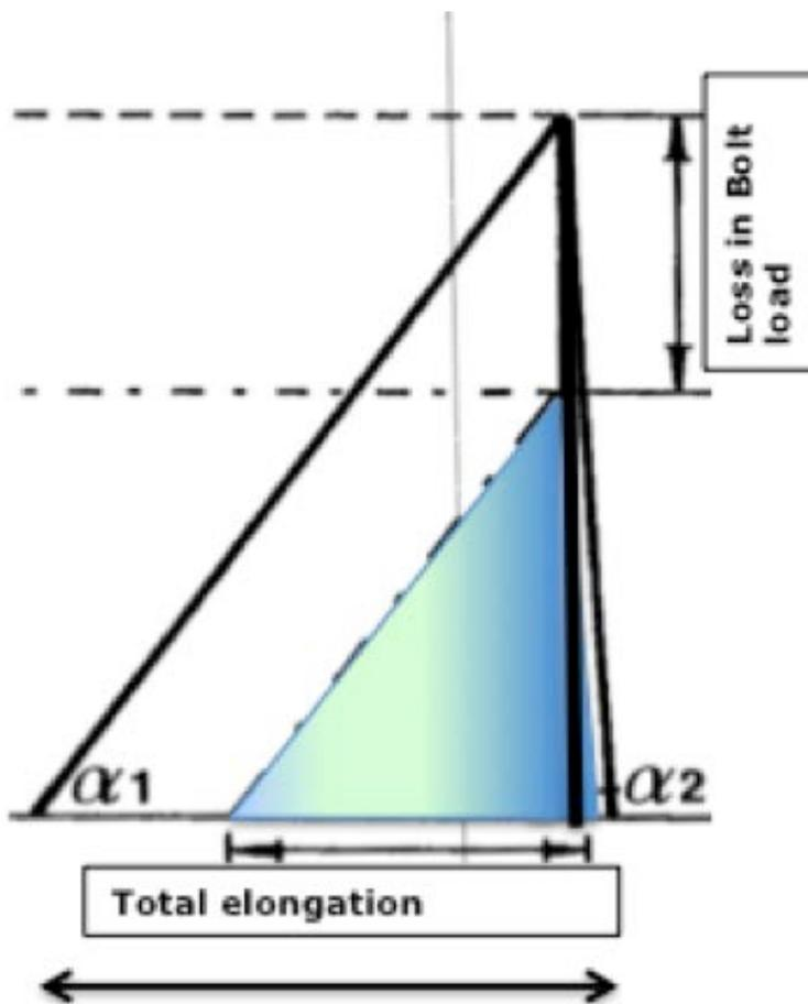
This triangular load diagram also helps to visualize the effect of relaxation, which results in loss of bolt load. The left part of the diagram relates to the elastic energy stored in the bolt while the right part relates to the cover.
