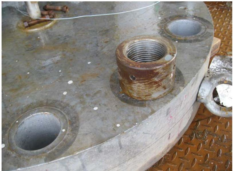
High relaxation may also result from dirt and from corrosion of the bolts, nuts and/or the contact faces of the cover.
