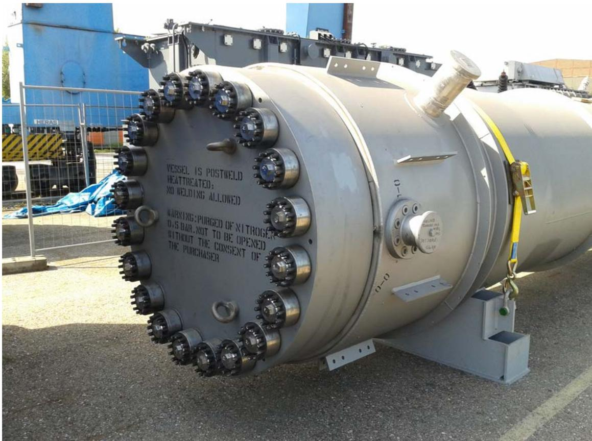
The picture shows the urea reactor with the superbolt design before shipment.
