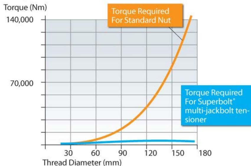
Also, with controlled lubrication and minimal frictional losses, superbolt reaches high preloads with superb accuracy and repeatability.
