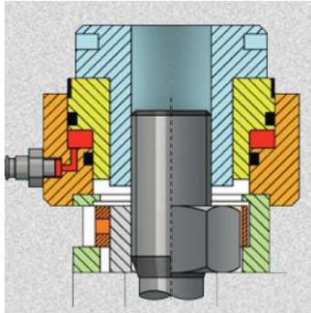
With this method, an axial tensile force is transmitted to the bolts with help of a hydraulic jack, which rest on the cover and is transferred to the bolt.
