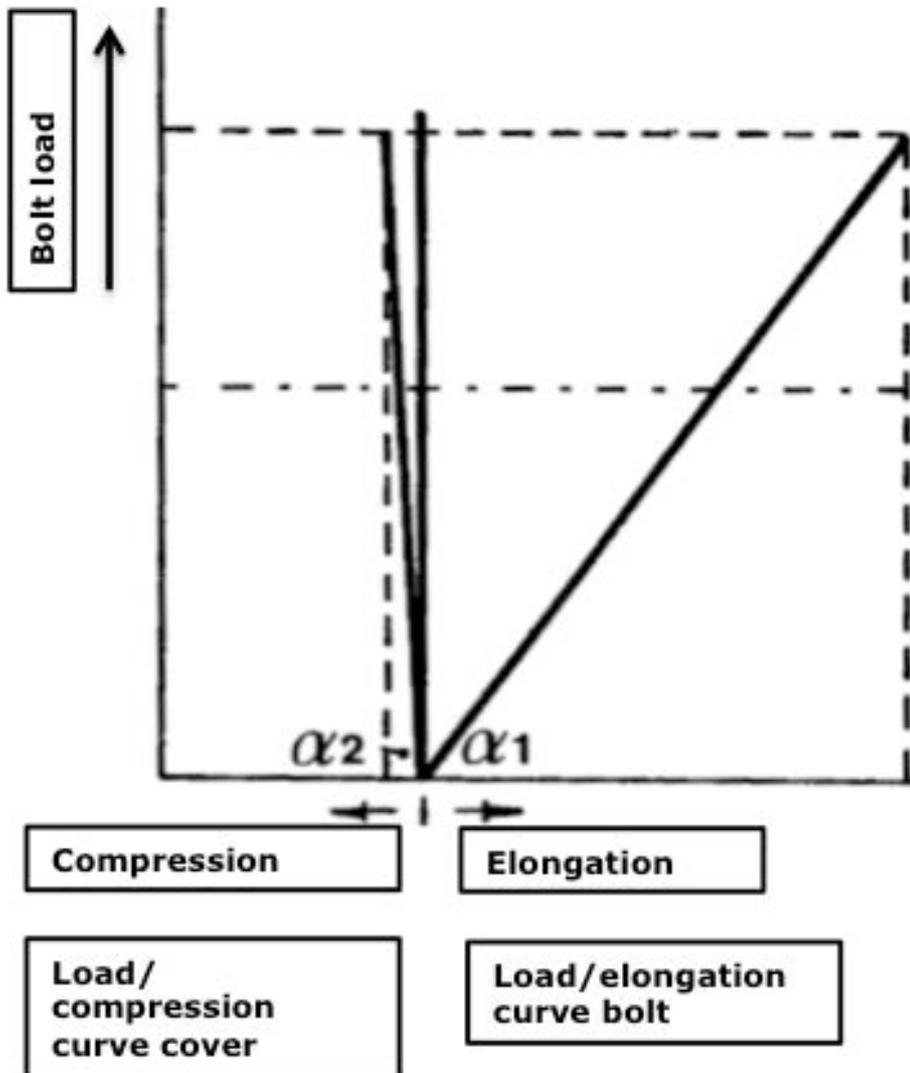
By moving the load/compression curve of the cover to the right hand side of the load/elongation curve of the bolts, a triangular load diagram is formed that shows the eventual elongation of the bolts.
