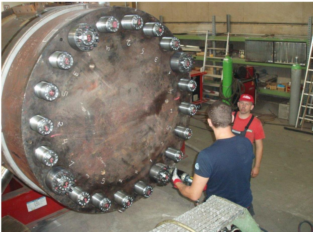
Reviewing the difference between conventional bolts and superbolts, we conclude that there is a significant gain in time to bolt up using superbolts in comparison to the hydraulic tightening with conventional bolts: Less than 50% of the time was only needed.
