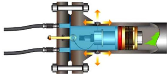
Figure 6. Hydrostatically testing with installed Reverse Pressure GripTight Test Plug
