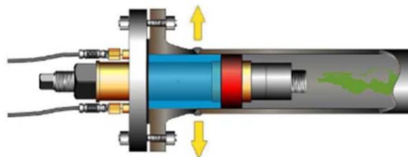
Figure 2. High Lift Flange Weld Test Plug in pipe
