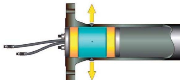
Figure 4. Double Block and Bleed Test Plug hydrostatic test
