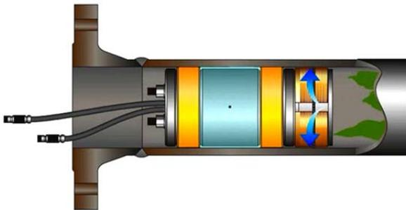
Figure 5. GripTight Isolation Plug
