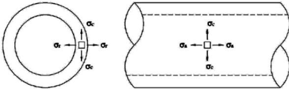
Figure 7. Stresses in a pipe
