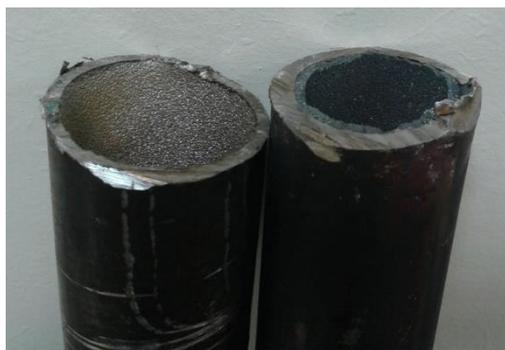
Photo 1 – typical fouling of the Urea Stripper
