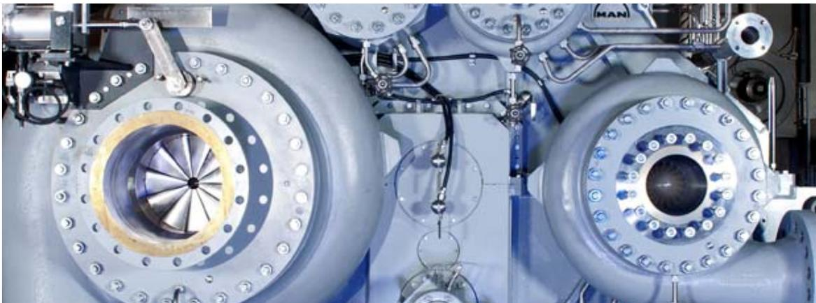
The integrally geared compressor is a multi-shaft centrifugal compressor. The number of stages is determined by the process requirements and the relationship between costs and efficiency. Typical
