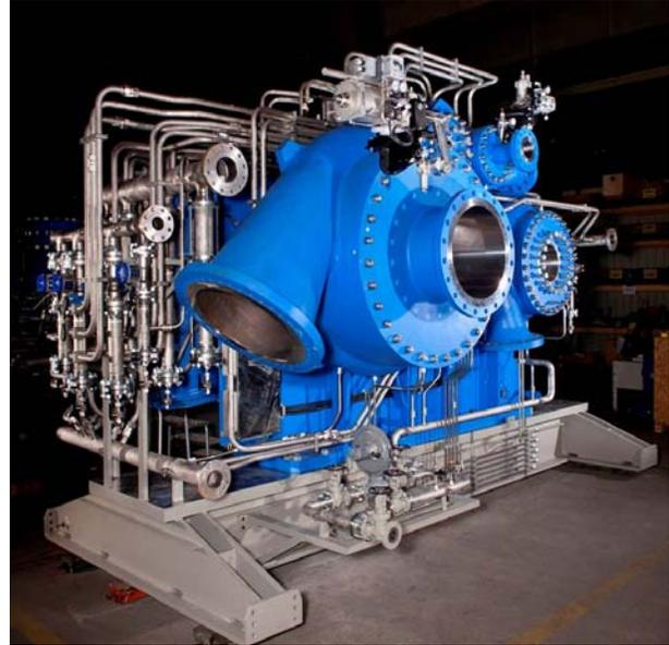
MAN Energy Solutions has unique compression solutions in its portfolio for the complete range of CO<sub>2</sub>, N<sub>2</sub>, propylene and vapour related applications, with single machines or complete train solutions. With accumulated **1 500 000 operating hours**, MAN is the world's number one in integrally geared CO<sub>2</sub> high-pressure applications, thanks to its sophisticated testing facilities and proven track records in the field.
