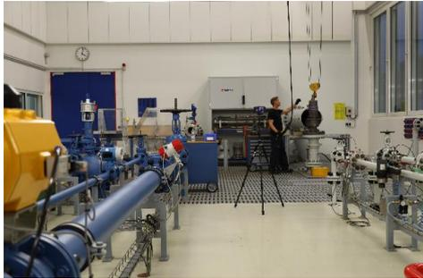
Safety valve being prepared for testing on LESER test lab
