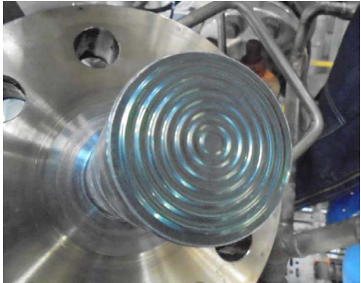
Figure 6: BADOTHERM Synthesis Pressure measurement
