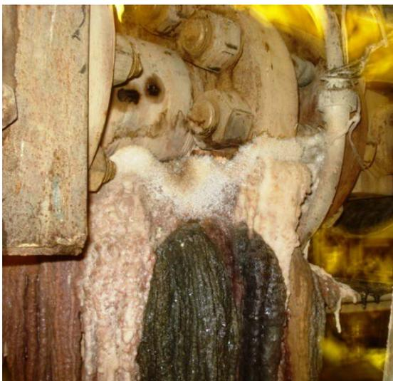
Fig (iii): Carbamate deposition with air sparge
