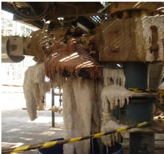
Fig (ii): Solid Carbamate mass encapsulating
