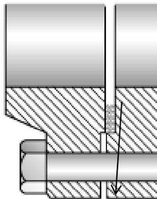
**Damaged Gasket of Male-Female Flange
