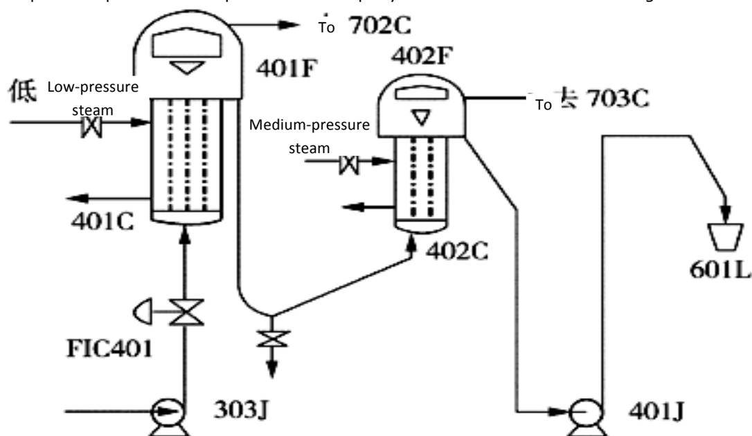
Figure 1: Flow scheme of the evaporation system
