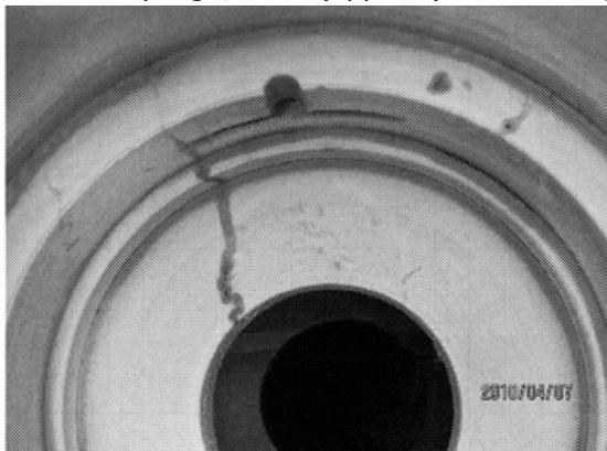
Fig.1 Crack in the valve cavity
