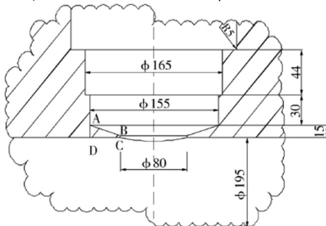
Fig.2 Structural diagram of valve cavity
