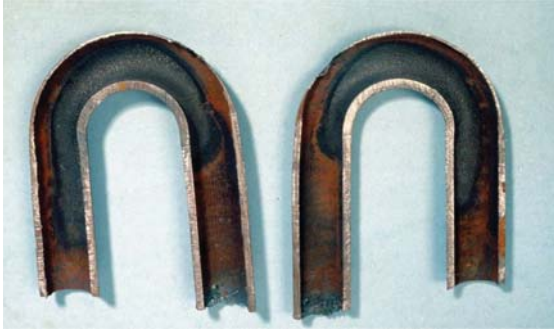
Figure 11 - Case 17: Erosion-corroded tube from a steaming economizer ( R = 0.68 ).
