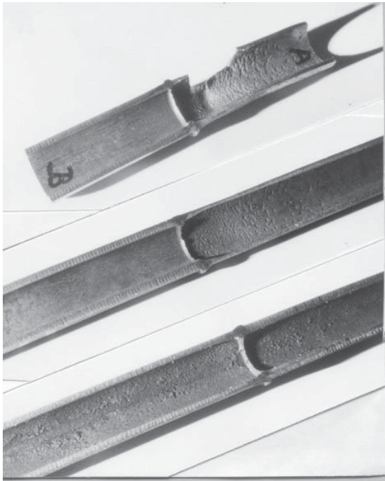
Figure 7 - Case 11: Tubes from the high pressure pre-heater. Erosion-corrosion downstream from the butt welds: (a) leakage ( R = 0.81 ), (b) erosion-corrosion ( R = 0.84 ), and (c) no erosion-corrosion ( R = 1.01 ).
