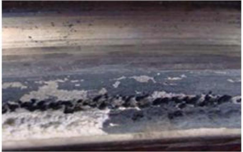
For example between a flange connection a crevice can exist when the two flanges are not connected in a correct way as shown in the figures above. In this crevice the carbamate solution is stagnant. Oxygen in the carbamate solution is slowly consumed because of the passive corrosion, after a certain period active corrosion will start leading to a leak and damage of the flange face.
