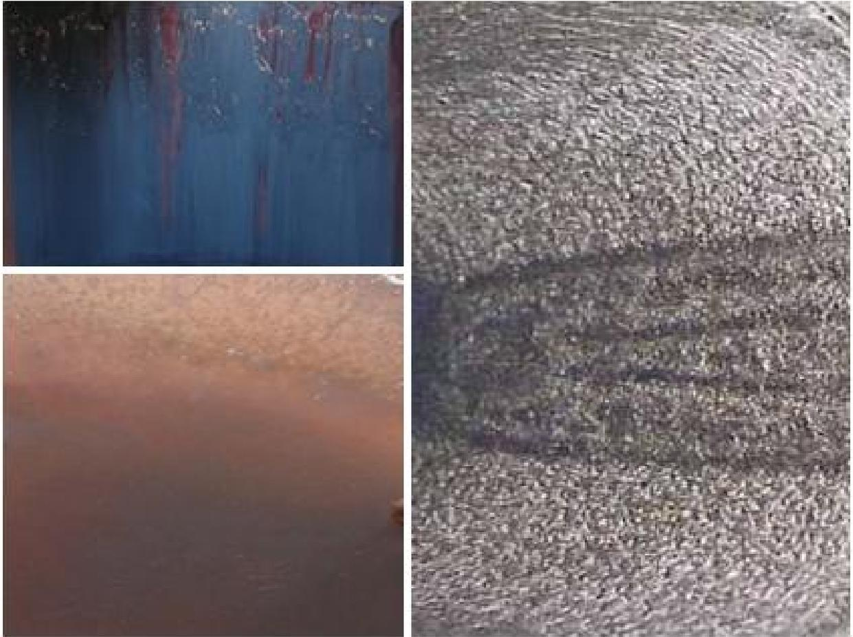
The pictures above show examples of passive and active corrosion in a urea plant. Passive corrosion (left) one can recognise by blue/reddish/brown colours indicating the oxygen layer. Active corrosion (right) however gives a shiny surface which is many times locally present, sometimes even with locally a significant reduction of the wall thickness.
