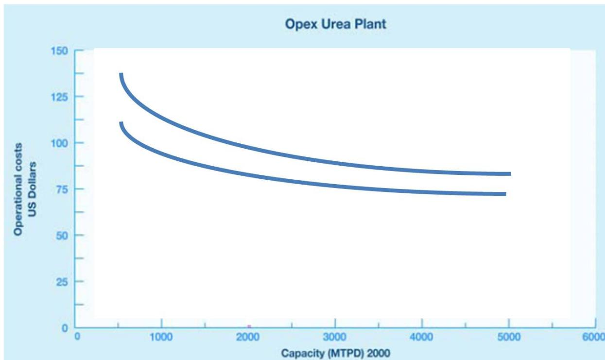
**Figure 1: Typical trend of range in operational costs versus plant capacity**
