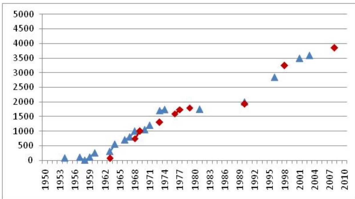
Figure 2: Maximum urea plant capacity licensed out in a certain year by either Stamicarbon (blue) or Saipem (red).
