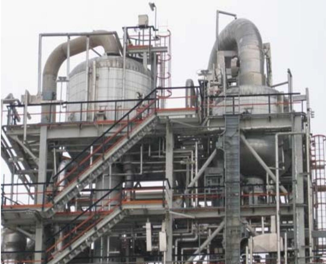
Figure 1: The heaters and separators of a two stage evaporation section
