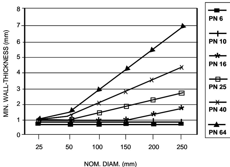
Figure 10: Required minimum wall thickness by weight and internal pressure.
