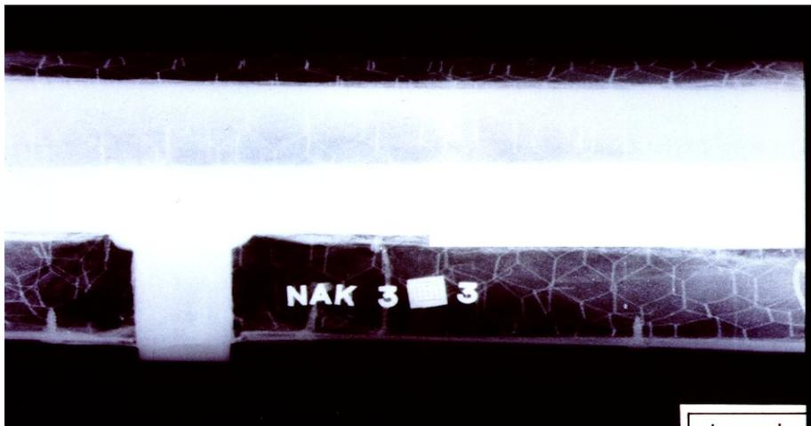
Photo 2: Picture of insulated pipeline taken with the aid of flash radiography
