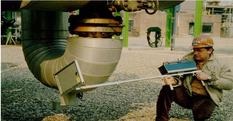
Photo 1: Inspection of insulated pipeline based on radiography technique
