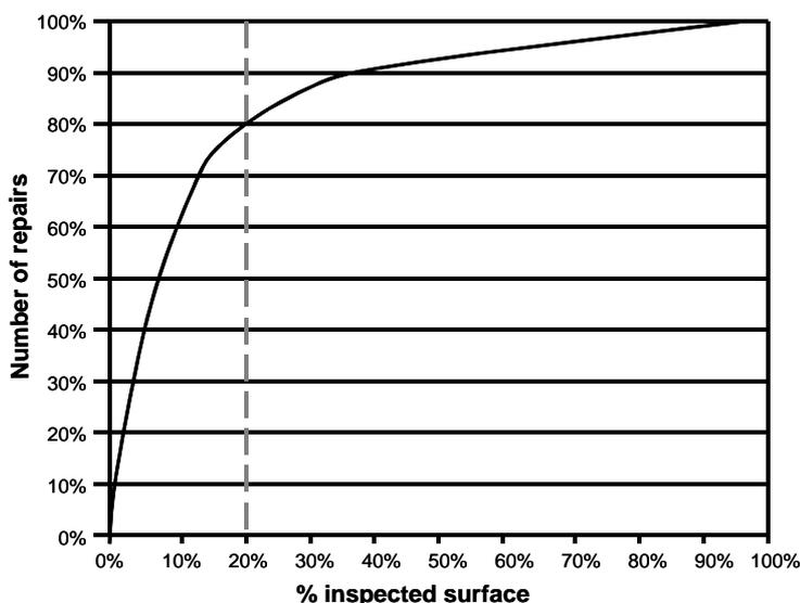
Figure 9: Repairs vs. inspections based on 13,000 measurements
