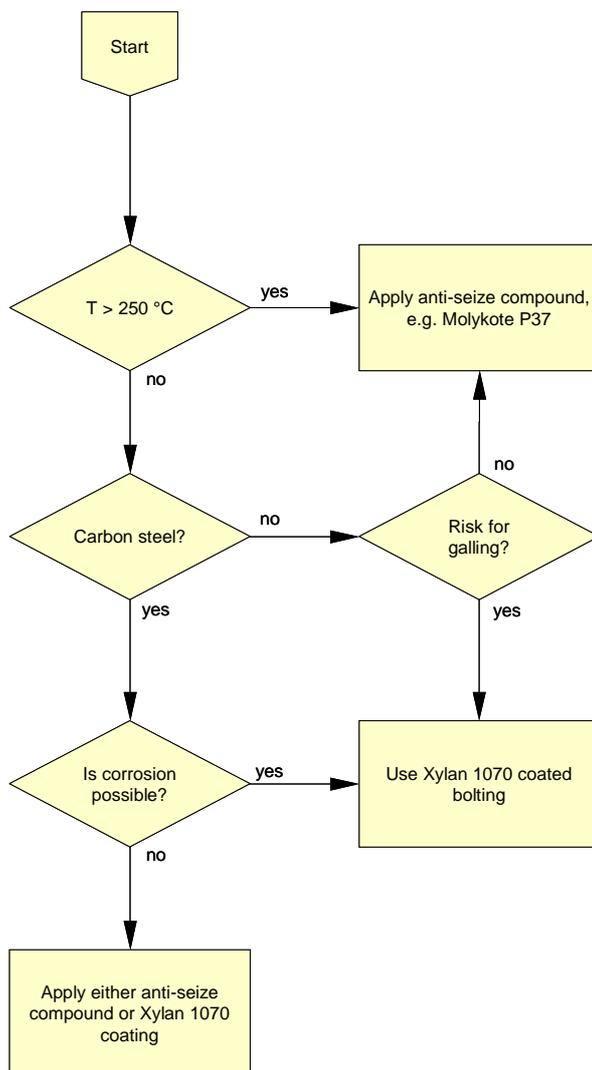
Figure 10: Selection chart for bolting protection
