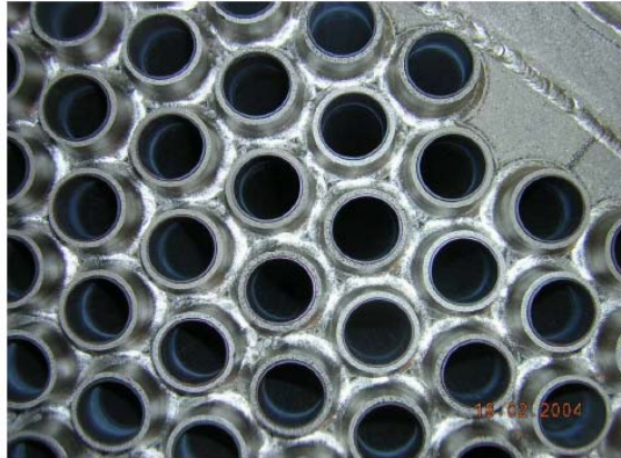
Corrosion at Tube sheet – Weld Overlay
