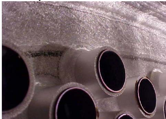
Corrosion at Tube sheet – Weld Overlay
