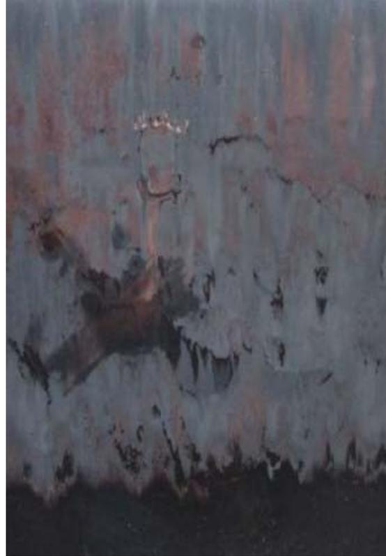
**Pictures: Bad insulation of a nozzle (left) can cause condensation corrosion (right)**
